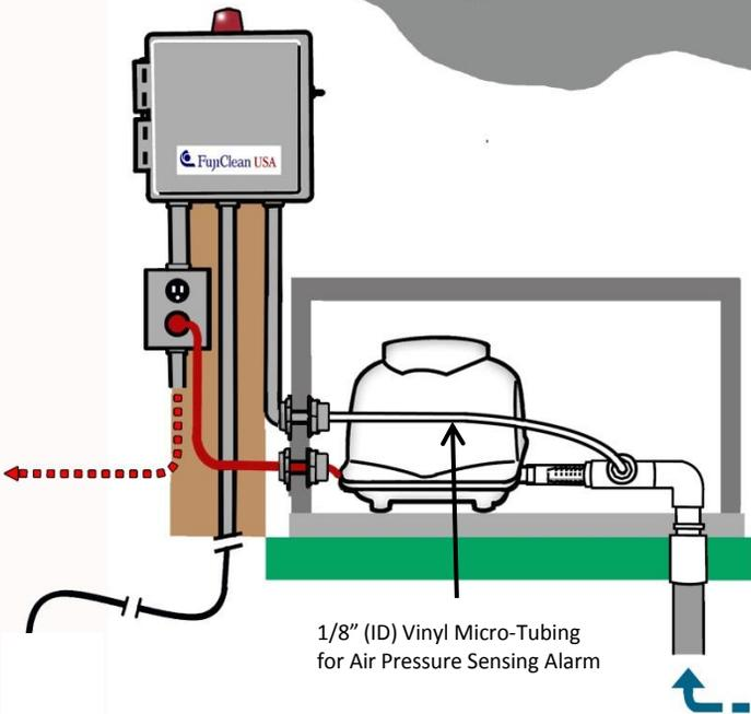
1/8" (ID) Vinyl Micro-Tubing for Air Pressure Sensing Alarm
