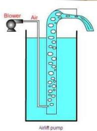
**Airlift Pumps.** This generic illustration shows the mechanics of the "airlift pumps" used in this system, which are simple pipe conduits through which pressurized air (from blower) is introduced at the bottom and by fluid pressure, water is carried up the pipe by ascending bubbles.
