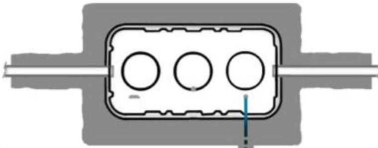
Plan view shows trench excavations for inlet and outlet lines
