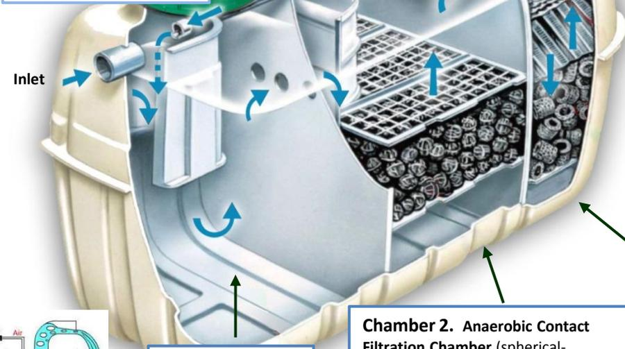
**Chamber 1. Sedimentation Chamber** (separates solids and greases)
