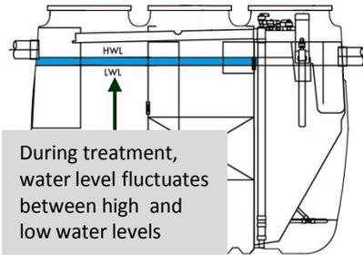
During treatment, water level fluctuates between high and low water levels
