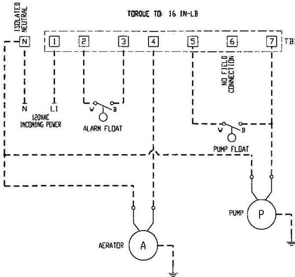
BRANCH CIRCUIT PROTECTION, OVERLOAD PROTECTION AND MAIN DISCONNECT PROVIDED BY OTHERS AND MUST BE SIZED ACCORDING TO PUMP/MOTOR MANUFACTURING SPECIFICATIONS.
