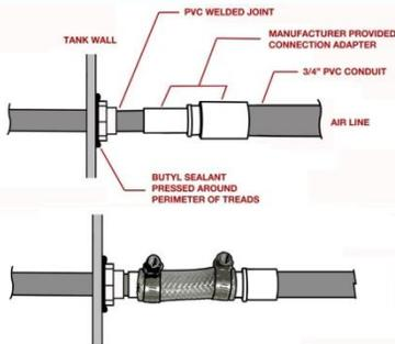
For connection air line to tank, use sealant meeting ASTM C990-96 standard to prevent septic gas transmission into control panel.
