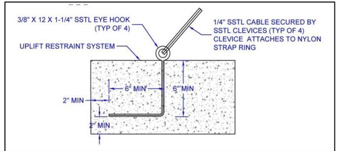
**Uplift Restraint with Concrete Collar**
