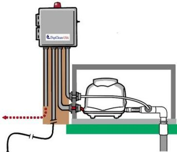
Note: Some states and installing contractors require hard wired blower connection
