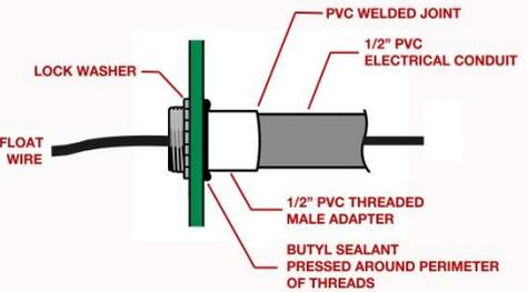
For connection of float switch cord to alarm panel, drill hole in riser and use male fitting and electrical conduit. Plug fitting with sealant standard that meets ASTM C990-96 to assure water-tight seal and to prevent septic gas transmission into control panel.
